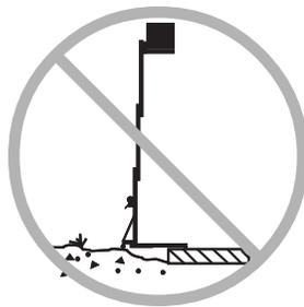
Do not raise the load unless the load handling attachment is properly secured to the machine.
