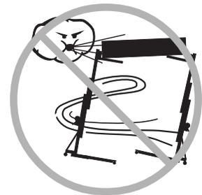
Do not leave a load raised when windy conditions may occur unless the machine(s) are properly guy-wired.
