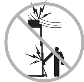
Keep away from the machine if it contacts energized power lines. Personnel must not touch or operate the machine until power lines are shut off.
