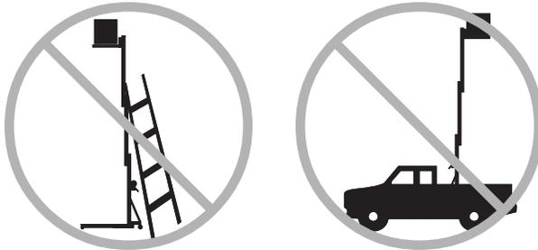
Do not use the machine on a moving or mobile surface or vehicle.
